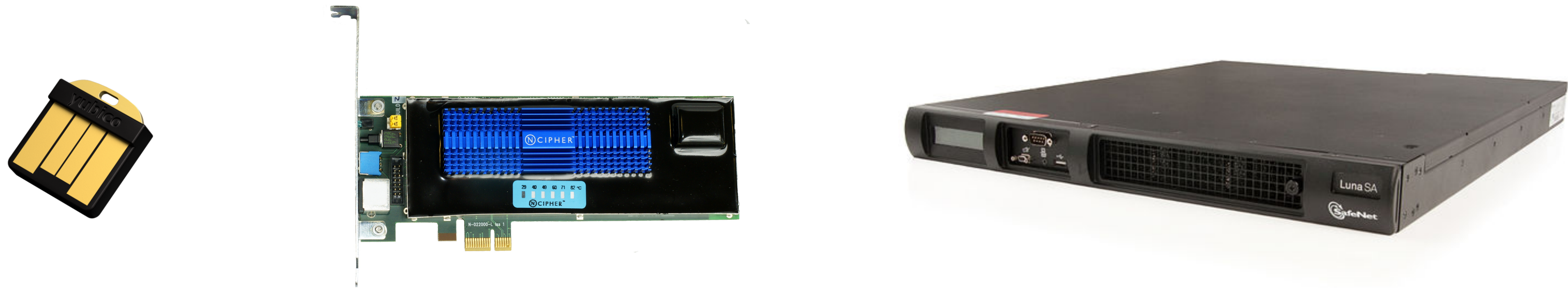
Hardware Security Modules
